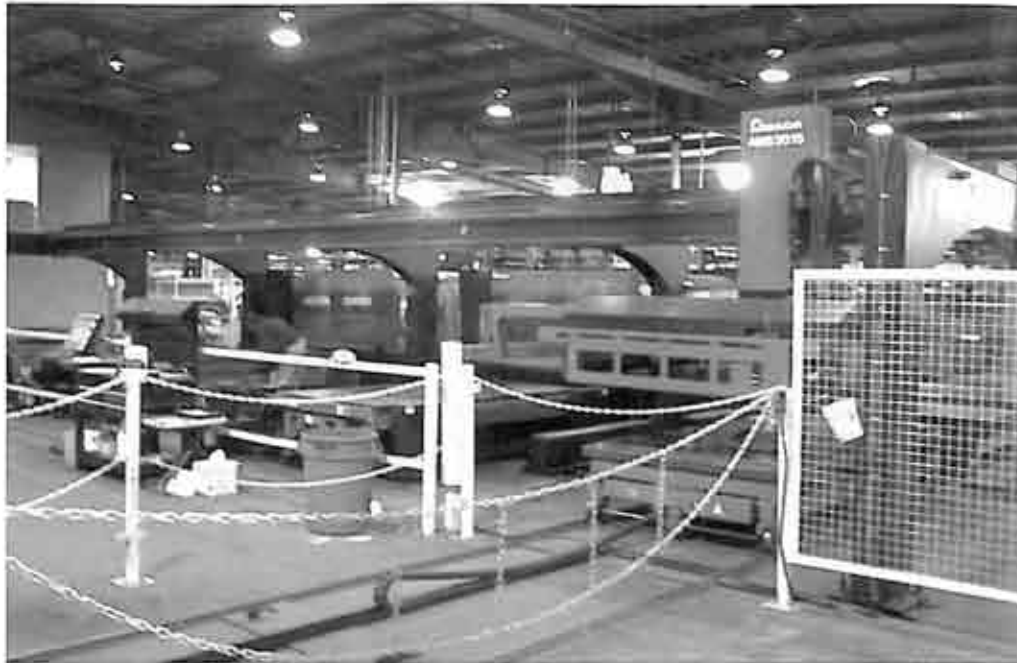
Above: A dual-laser cell with loader/unloader at Kasa Fab in Salina, Kansas.
