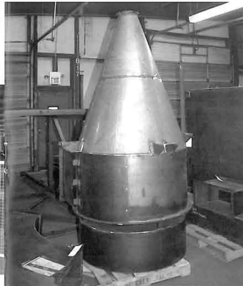
Above: A large hopper fabricated at Kasa Fab.
